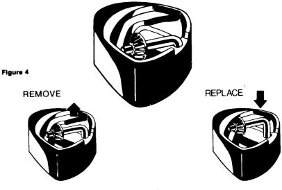
To remove the chuck from the Drill, for using a threaded shank accessory or for chuck replacement, open the chuck and remove screw in bottom of chuck (left hand thread). Insert the key in the chuck and tap it sharply in the direction the tool normally rotates — see at right. This will loosen the chuck shank threads and the chuck may be unscrewed by hand (See Figure 5).
